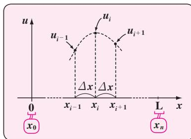
$$\begin{aligned} \text{(①の左辺)} &\doteq \frac{\overset{\text{新時刻}}{u_i} - \overset{\text{旧時刻}}{u_i}}{\Delta t} \dots\dots \textcircled{3} \end{aligned}$$
